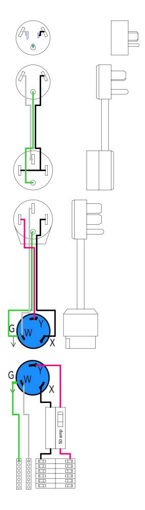
Adapters to attach 50 amp RV to 15 amp outlet
