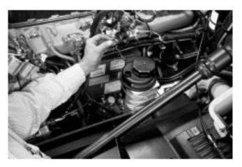
Check all fluid levels. Make sure there are no signs of leakage after changing oils or filters.
