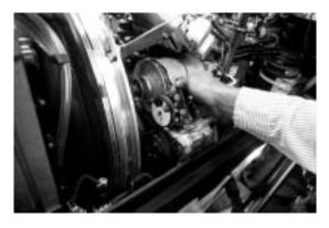
**36** Check Alternator Mounting and Electrical Connections
