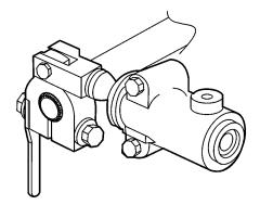
Fig. 2: Volvo Clutch Slave Cylinder
